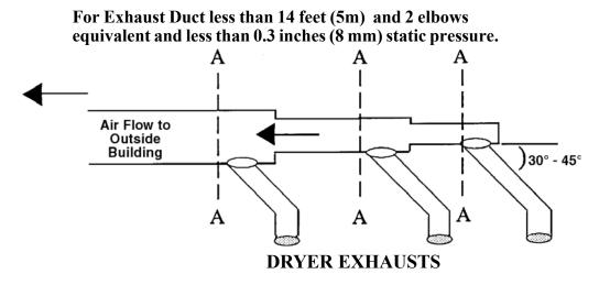
Area of section "A-A" must be equal to the sum of dryer exhaust pipes entering multiple exhaust pipe. (See chart below.)
