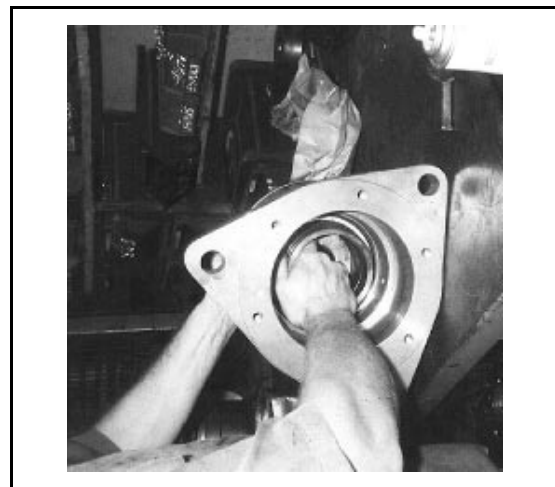
FIGURE 6 (MSSM0303AE) Installing Seal Sleeve in Bearing Housing
